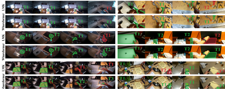
Fig. 5: Qualitative comparison for challenging scenarios. We compare LMK and Whareformer on HD-EPIC (left) and IT3DEgo (right). Top: Whareformer maintains consistent track identities through pick-and-place motions (left) and motion blur (right). Middle: Whareformer successfully disambiguates spatially close objects without merging tracks. Bottom: Whareformer maintains precision in clutter (left) and sustains identity during long-distance room transits (right).
